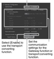
Input the IP address of the target CNA-1 for the transport converting function.
