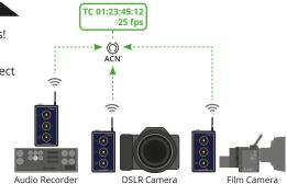
Timecode from an external source can now be sent from one device to other devices.
