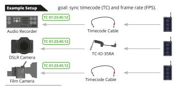
NOTE: Required cable depends on connected device. E.g. TC-IO for ARRI, LTC-Out/Epic for RED, LTC-Out for BMD. Canon. Panasonic. Sonv. Please check our website.
