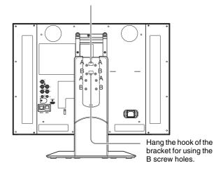
**5** Secure the arm with four screws.
