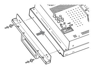
**2** Attach the unit to the rack with four screws.
