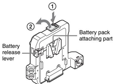
Insert the projection of the battery adaptor into the slot on the rear of the camcorder (①), then lower the ejection lever (②).
